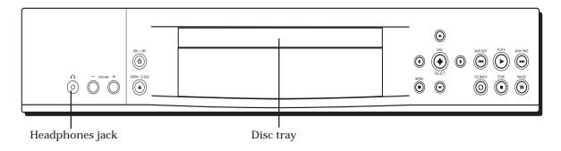
Disc Tray Press OPEN • CLOSE to open and close the disc tray.
